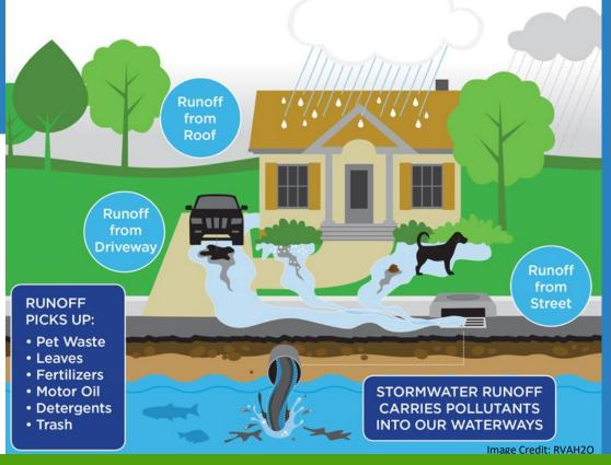
Stormwater pollution is the uncontrolled runoff of rainwater from hard surfaces such as roofs. driveways, roadways, parking lots and even lawn areas. This water enters our storm sewer system where it is discharged untreated to our local creeks contributing to impairment.
