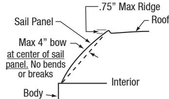
**SAIL PANELS:** Must slope down from rear edge of roof and extend from roof to deck and be the same on both sides. May extend 2" maximum past rear edge of interior deck.
