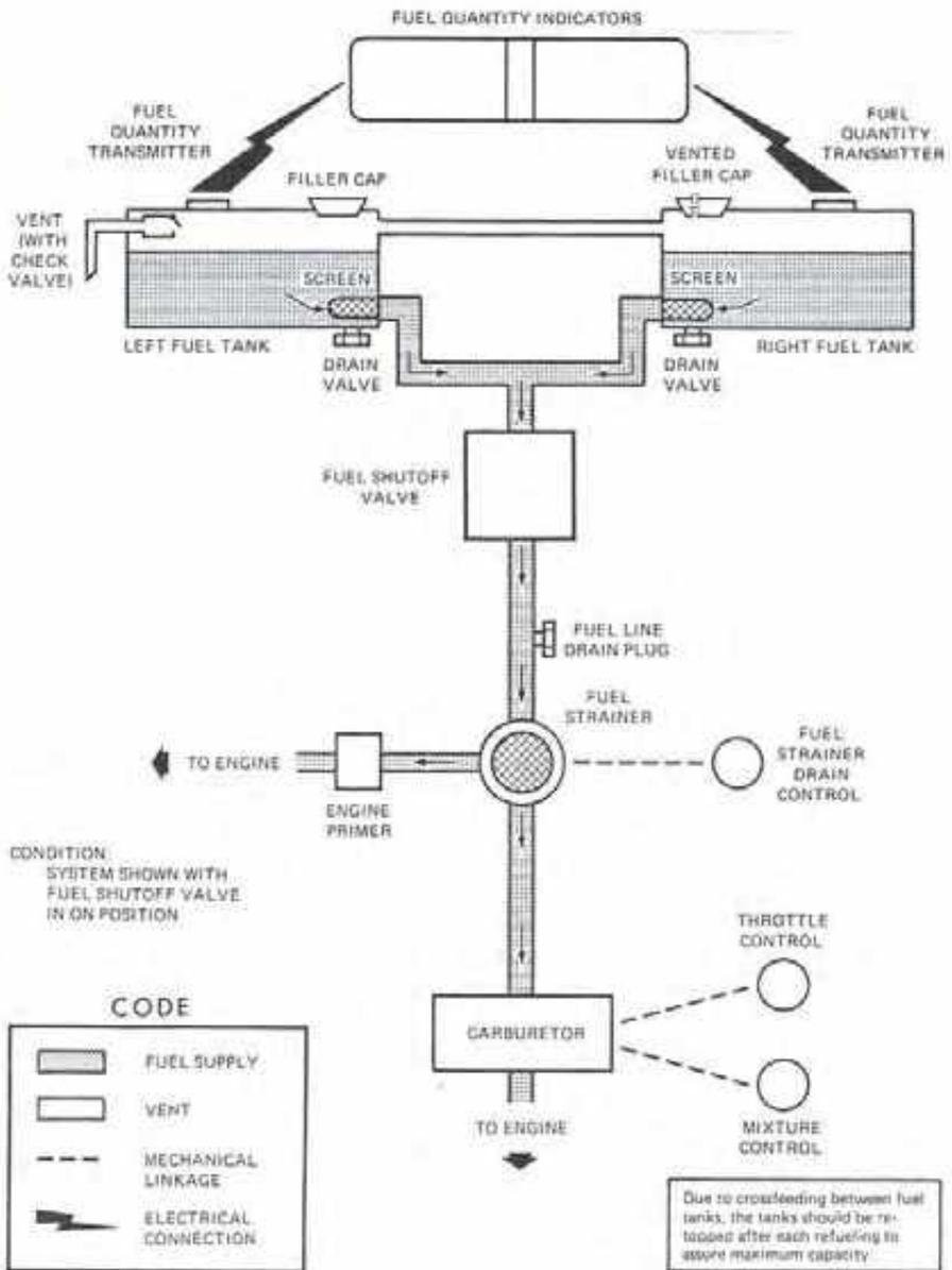
Figure 7-6. Fuel System (Standard and Long Range)
