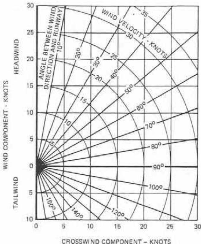
Figure 5-4. Wind Components
