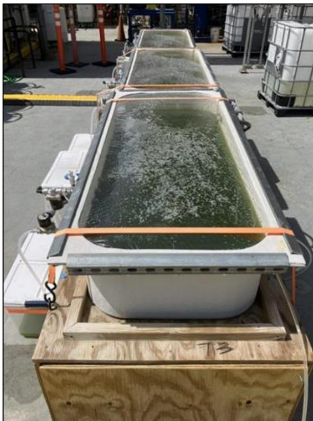
Figure 16: Integrated MSC system at NCCC bench-scale site (photo John Carroll, NCCC)
