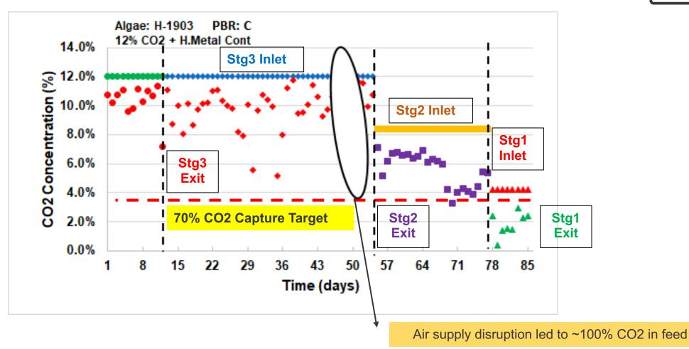
Fluctuating light intensity results in varying exit CO<sub>2</sub> concentration in the respective stages
