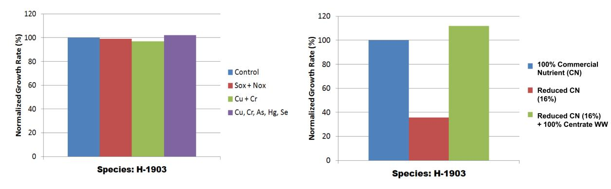
• Algae tolerance to key post-FGD flue gas contaminants demonstrated
