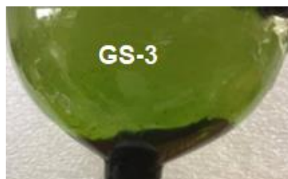
Figure 13: Settled algae at conical bottom of GS-3 (Confidential)
