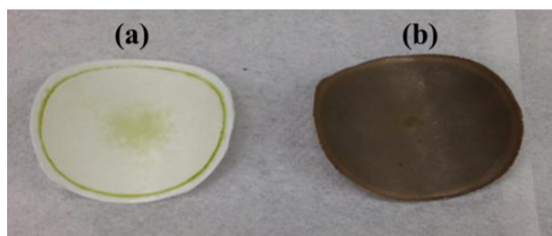
Figure 17: Images of (a) an uncoated and (b) a PEG+PDA coated PSf-100 after algae dewatering test with the algae concentration of 35.8 g/L. (Confidential)
