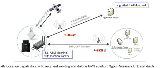
4G Location capabilities – To augment existing standalone GPS solution, 3gpp Release 9 LTE standards adds commercial MS-assisted and MS-based aGPS, Observed Time Difference of Arrival (OTDOA), and Enhanced Cell ID solutions (using 4G SUPL). OEMs can also use these and Hybrid (combination of methodology) to allow for better location for indoor and/or outdoor environments than standalone or legacy techniques (e.g. 3G-based, Cell ID, etc.).
