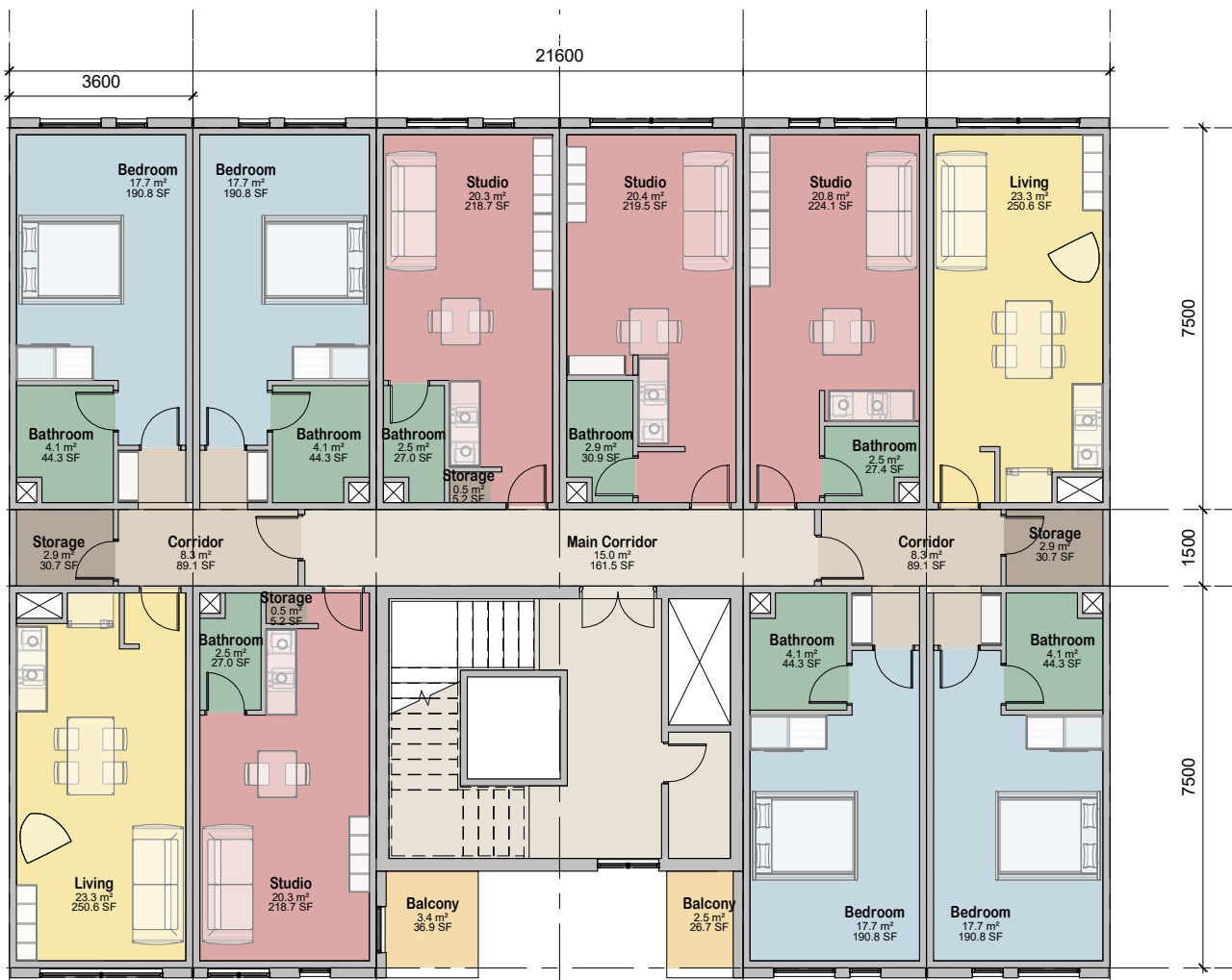
Fig.34 Conceptual building layout for infill building no 1 _ Floor plan / out of scale
