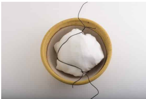
Second pair of wires connected close to the other hole with one wire
