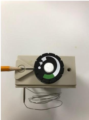
With the cover reinstalled the knob is in the off position. This is directly in line with the spark button location. Please mark the raised bar with a felt pen for future reference.
