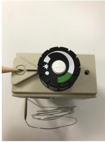
Turn to knob to the spark position as indicated. Press down and spark till the pilot is lit. Release and ensure pilot is staying lit. **\*\*important\*\* if not repeat.** Once pilot is established proceed to next lighting the burner
