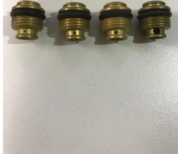
You can see drill holes of the bypass screws here vary in size. It is important to confirm.
