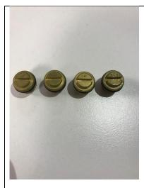
There are many different jet sizes of the bypass screw. Each is stamped on the top with a number, 60, 100, 120, 190, 240.
