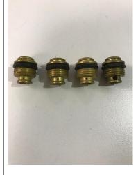
You can see drill holes of the bypass screws here varry in size. It is important to confirm. As the AGA control is a specialzed modulating control valve. This means on high fire it uses 15,000 BTU of fuel. On its lowest setting it uses 6,000 BTU of fuel. The control modulates between both these setting as need to restore heat to the cast iron as needed.
