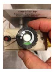
You can see that the dot on the control is in line with the raised black line leading to the spark button. (We have marked this with a felt tip marker yours may not be marked black)
