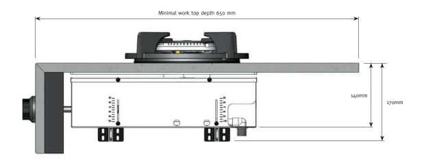
Front Side can be applied to the front side of the work top as well as the blind of the kitchen cabinet (whether indented or not). The designs above show the required measurements. The center-to-center measurement of the knobs depends on the situation, and the C-measurement is fixed.
