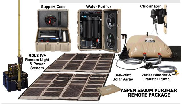
The Aspen 5500M water purification system will supply 4,000-5,500 gallons (approx. 15,000-20,000 liters) per day of highly purified water from virtually any non-saline water source. Water can be drawn from ditches, rivers, lakes or standing water that may contain chemical and/or biological contamination. The purifier has its own built-in solar charging controller and storage battery to run 6 to 8 hours a day off of solar.
