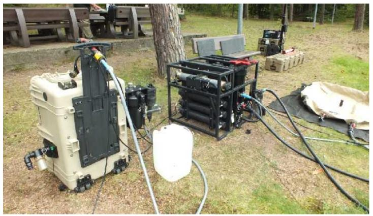
Aspen 3300M (Fresh Water Purifier) in Tan with Chlorinator and Aspen 1000DM ROWPU, Fresh to Seawater system. All equipment including Lights ran on the 2000 Watt Generator located in the base of the light package. Solar array was also demonstrated on the Aspen 3300M
