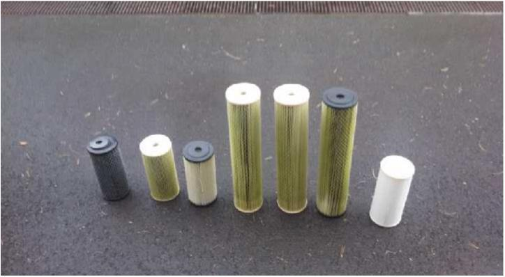
Water taste equal to Bottle Water. Prefilters show algae and other matter removed from pond prior to water treatment. These filters can be cleaned and reused. The dark Grey post-filter color was unchanged.
