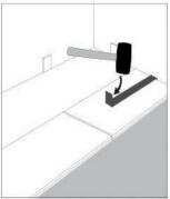
to lock final piece in row. Insert spacer at end of row. Continue installation to final row.
