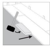
Step 5: IMPORTANT! Use a hammer and tapping block to tap the long edge of the plank to ensure a tight fit. Note: Tapping block should be a minimum of 10" to 12" long. It is important to note that any/all gapping can/will compromise the locking system.
