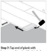
hammer and tapping block to lock ends of planks together. Remove support bridge and continue with this Step 8: Use hammer and pull bar method until you have completed installing the row. Note: BE SURE TO TAP ON EDGE OF VINYL SO AS NOT TO DAMAGE LOCKING PROFILE.
