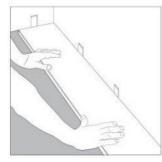
Step 1: Begin installation working from left to right. Insert 6-10mm wide spacers at ends and edges where planks meet wall.
