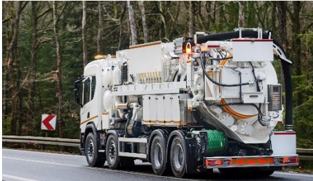
Sewer cleaning equipment
