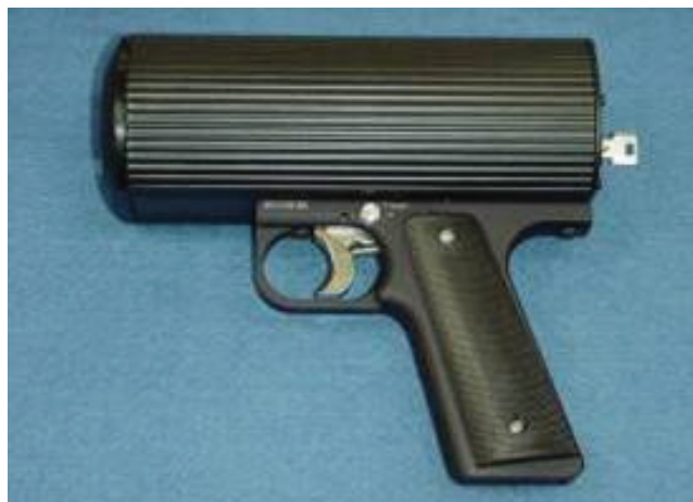
FIGURE 7 Laser used for dispersing birds (Source: USDA/APHIS/WS Ohio Field Station).
