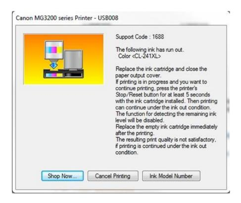
Notice this message asks you to hold the printer's "STOP" button for 5 seconds, we recommend holding the "STOP" button until the message disappears. Follow these instructions and you can continue printing without difficulty.
