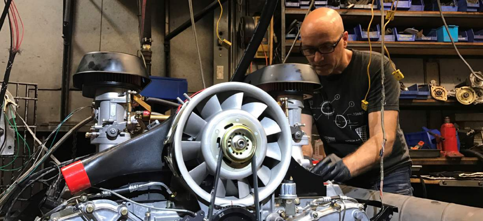
Working in the Hasselgren dyno - 3.2 L short stroke 911 engine
