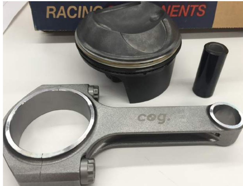
Raimond's custom designed piston, connecting rod, and wrist pin (DLC coated)
