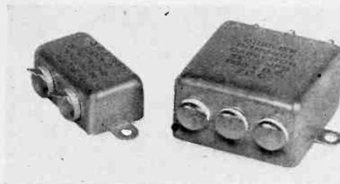
Under chassis type Dubilier Nitrogol condensers with side contacts and ceramic insulation. This is a tropical style suitable for use under conditions of high ambient temperatures.
