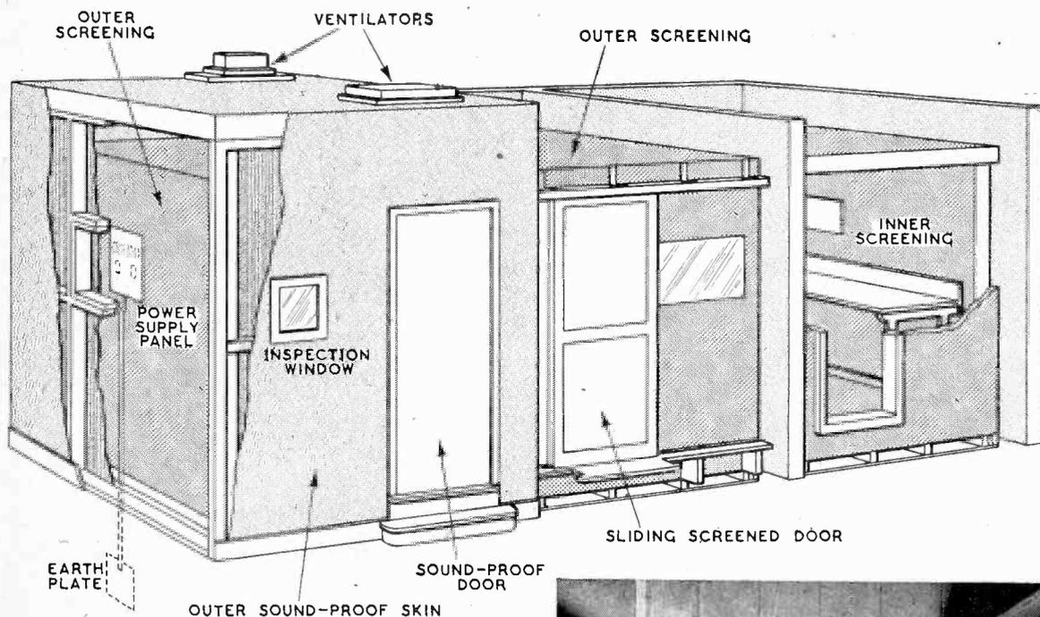
also be seen the two rails on which the doors run, the tapered copper-covered floor ramp, and the contact springs on the leading edge of the doors. There is also an outer hinged door to complete the acoustic screening.
