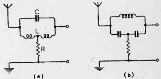
paid for somehow; at the frequency of the wanted signal there is a small loss of energy due to the presence of the short resistance. We shall see, however, that the resistance value is of the order of 10,000 to 100,000 ohms; the loss introduced is therefore very small.
