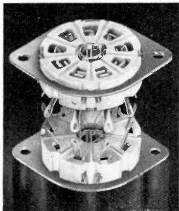
Top and bottom views of "Clix" type B9G valve-holder for all-glass valves. The sockets are anchored to minimise the risk of flash-over between pins or breakage through misalignment.
