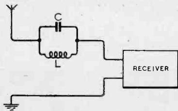
Fig. 1. Conventional wavetrapp circuit text-book device, although actually it is a simple and practical circuit.
