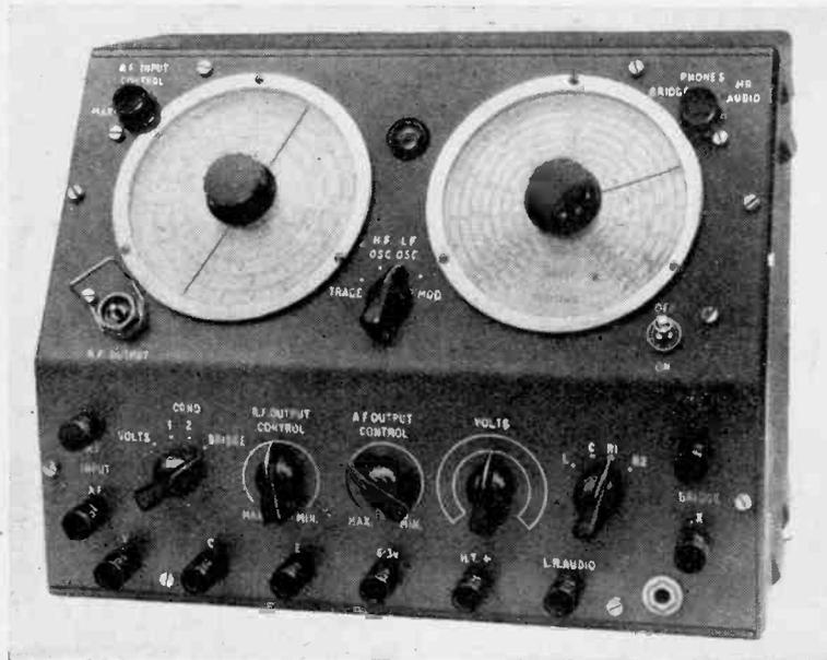
Labgear "Electronic Fault Tracer" for general testing and service work.
