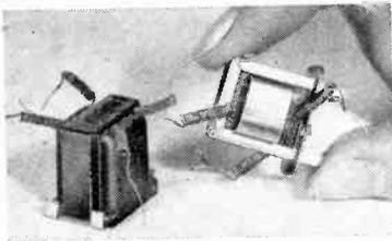
Good response over the essential speech frequency band is claimed for these midget AF transformers made by Bulgin. Bakelite cased and open types are available.
