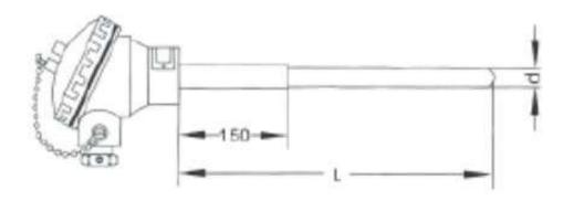
Protection Tube Material: Stainless Steel, Corundum Available Diameters: Φ16 mm, Φ20 mm, Φ25 mm, Φ32 mm Tube Length: Customizable based on application requirements
