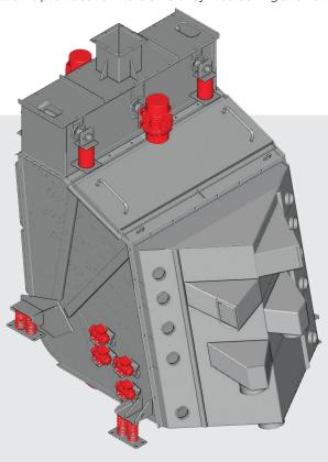
Spreader feeder for even distribution over width.
