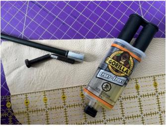
Apply epoxy to the cut end of the  $\frac{1}{4}$ " bolt and insert the other half of the bolt into the  $\frac{5}{16}$ " brake line and allow to dry.
