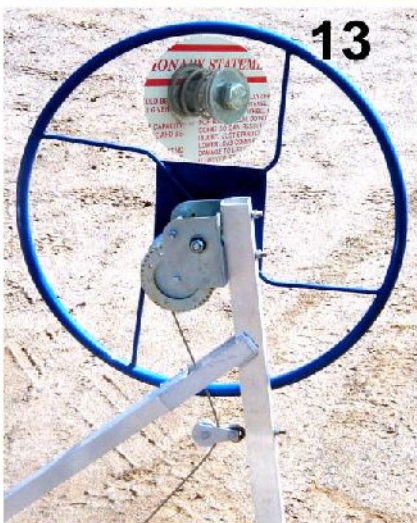
13. mount the operators wheel follow the instructions included in the yellow winch instruction sheets.
