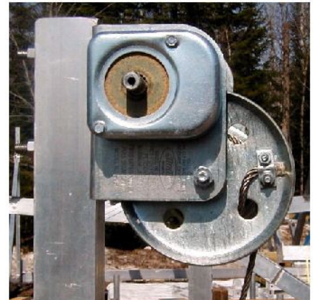
12. mount the cable to the winch, follow the instructions included in the yellow winch instruction sheets.
