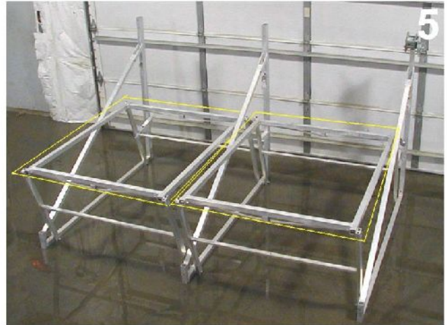
5. place the top frame at the un-bolted ends of the H-frame the 2" x 3" tube should be on the bottom when it is set in place
