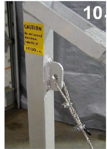
10. un-coil the cable, wrap one end as shown thru the welded pulley tab mount the cable clamps and tighten them.
