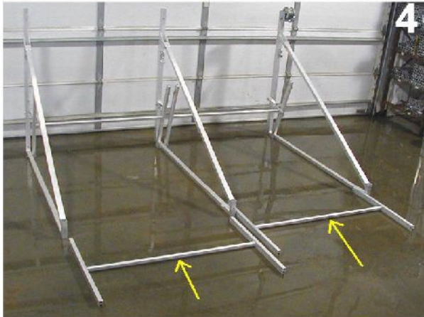
4. mount the 3rd & 4th H-frames to the water end of the lift. Use page 2 Details C,D&E for the bolting detail, the bolts are the same.
