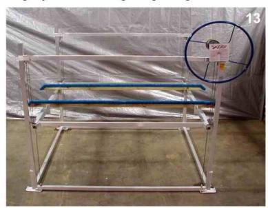
13,14&15. Mount cradles as shown using 1/4" nuts, bolts and washers. The cradles will need to be adjusted to your watercrafts hull when the boat lift is installed.
