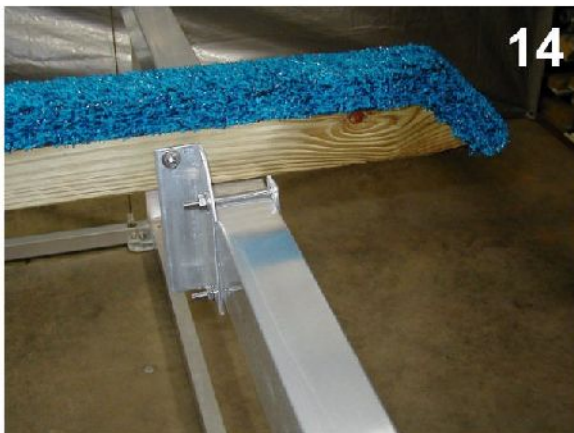
13 & 14. The cradle hardware is all in one bag. Bolt the Cradles to the top frame as shown install watercraft and position the cradles before raising the lift adjust to fit and then tighten the cradle hardware. Now tighten all the lift nuts and bolts. Do not over tighten the bolts (snug is good) they are easy to over tighten.
