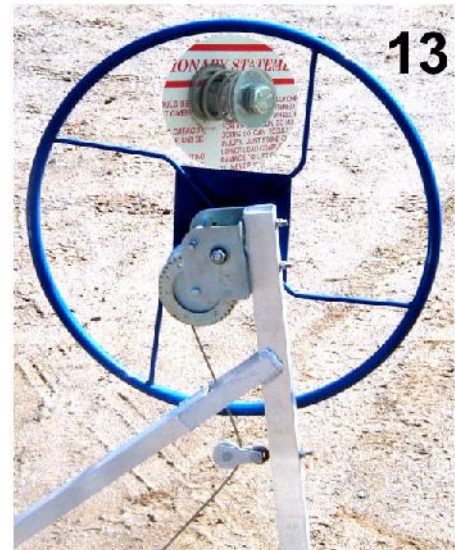
11. string the cable thru the 3 pullies as shown
