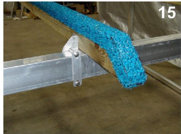
13 & 14. The cradle hardware is all in one bag. Bolt the Cradles to the top frame as shown install watercraft and position the cradles before raising the lift adjust to fit and then tighten the cradle hardware. Now tighten all the lift nuts and bolts. Do not over tighten the bolts (snug is good) they are easy to over tighten.
