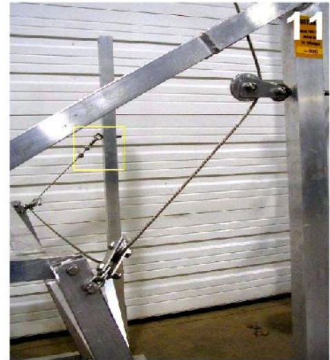
11. string the cable thru the 3 pullies as shown
