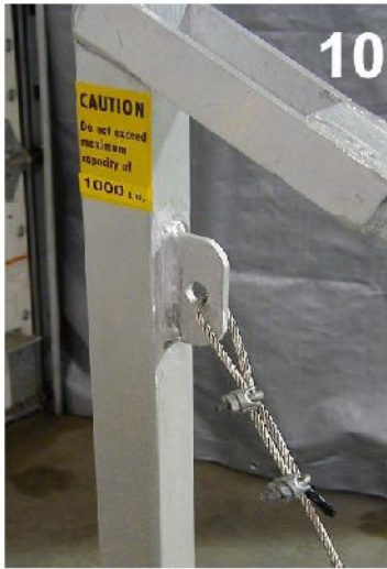
10. un-coil the cable, wrap one end as shown thru the welded pulley tab mount the cable clamps and tighten them.
