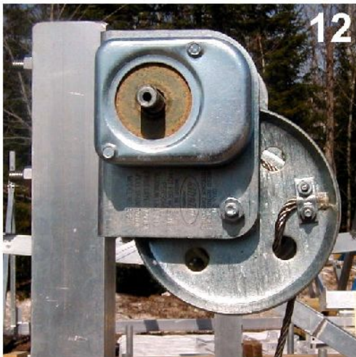
12. mount the cable to the winch, follow the instructions included in the yellow winch package
