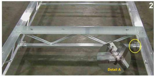
Warning: Donot over tighten Bolts, this may cause the nuts to lock up.
