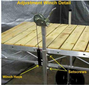
Dock Adjustment: Slide winch over the axle leg post, place the Winch Hook under the leg bracket and crank up winch to remove excess slack from the lifting cable. Loosen the Setscrews on the axle leg bracket and lower the Dock about 1" to create slack in the "X" cables, feed the necessary number of chain links thru the chain bracket ear, see (Detail D and E) Adjust the Dock to the correct height. (Adjust each side no more than 10" at a time or binding may result.)
