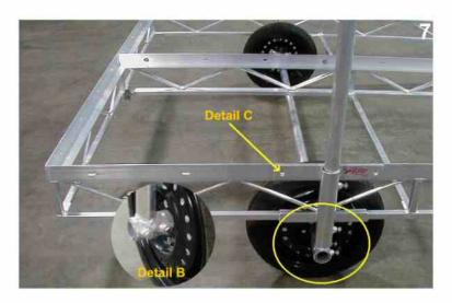
5&6. Slip the axle leg bracket over the axle leg
