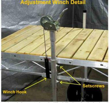
Dock Adjustment: Slide winch over the axle leg post, place the Winch Hook under the leg bracket and crank up winch to remove excess slack from the winch cable. Loosen the Setscrews on the axle leg bracket and lower the Dock about 1" to create slack in the "X" cables, feed the necessary number of chain links thru the chain bracket ear, see (Detail D and E) Adjust the Dock to the correct height. (Adjust each side no more than 10" at a time or binding may result.)
