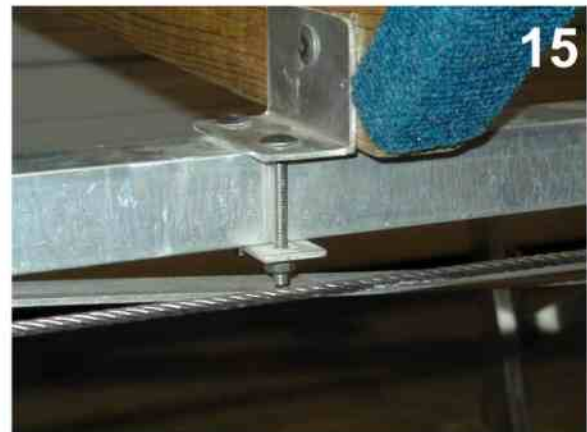
13 & 14. The cradle hardware is all in one bag . to the top frame as shown install watercraft and position the cradles before raising the lift adjust to fit and then tighten the cradle hardware. Now tighten all the lift nuts and bolts. Do not over tighten the bolts (snug is good) they are easy to over tighten. PAGE 4 OF 4
