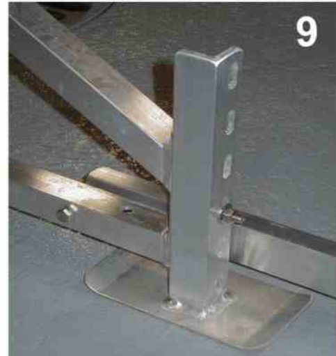
9. Mount the foot pads on the rear of the lift using 3/8 x 3 cap screws use a washer in the foot pad side of the assembly
