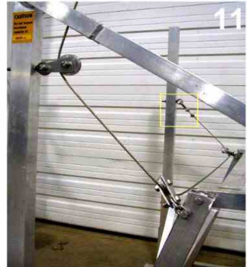
11. string the cable thru the 3 pulleys as shown
