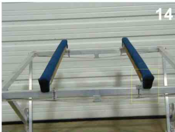
13 & 14. The cradle hardware is all in one bag . to the top frame as shown install watercraft and position the cradles before raising the lift adjust to fit and then tighten the cradle hardware. Now tighten all the lift nuts and bolts. Do not over tighten the bolts (snug is good) they are easy to over tighten. PAGE 4 OF 4
