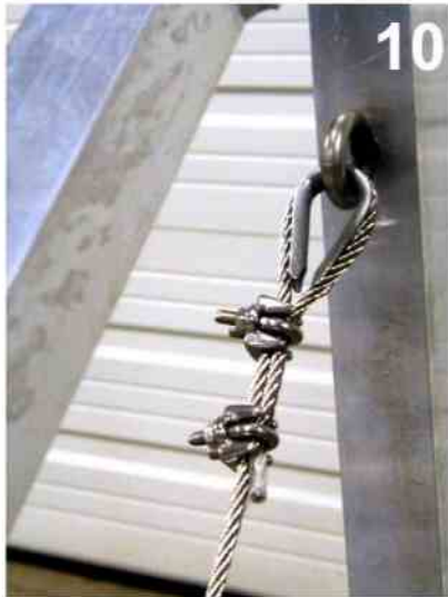
10. un-coil the cable, wrap one end as shown thru the eye-bolt using the cable thimble at the eye-bolt to protect the cable. mount the cable clamps and tighten them.
