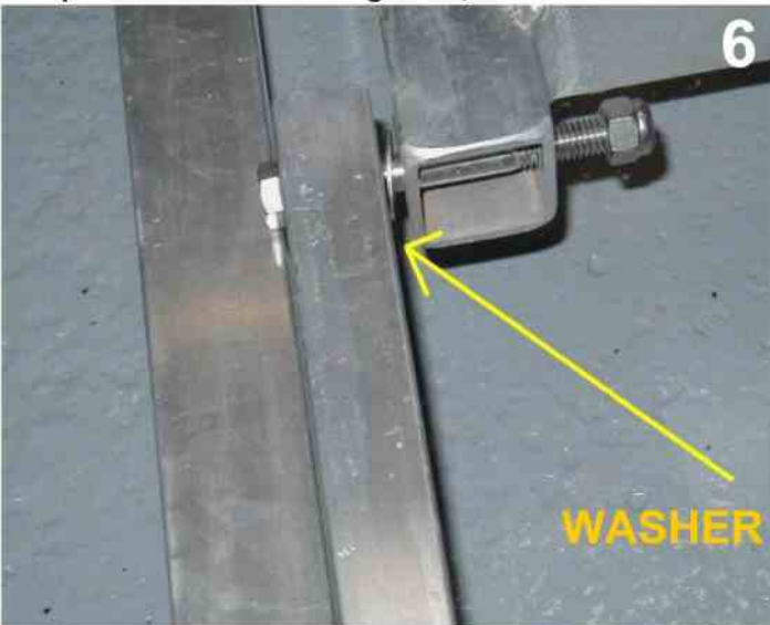
6. bolt the top frame to the H-frame ends using 4-3/8 x 3 1/2 cap screws washers and nylon locknuts Note the placement of the washer.
