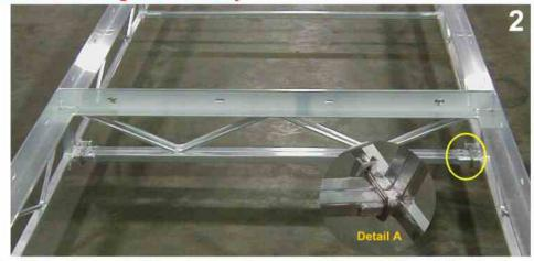
(Floats should be mounted first) The frame bolting instructions are shown without floats for clarity Warning: Donot over tighten Bolts, this may cause the nuts to lock up.
