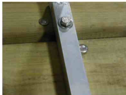
Remove mounting pad and mount under deck with 1/4" x 2 1/2" CB. nuts and washers. Secure ladder to plate with 3/8" x 3" cap screws.
