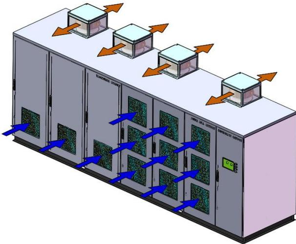
Sketch of optional duct for extracted air
