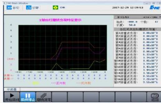
Simulation display and evaluation of the screw status using the CNC system interface and corresponding algorithms.
