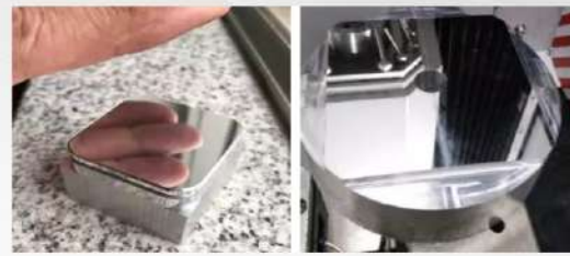
High precision finishing to achieve a high gloss surface
