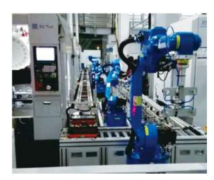
♦ The is the 2016 demonstration project of new manufacture standardization shown by the Ministry of industry and information technology. This project includes 200 sets of Huashu high speed drilling and tapping equipments, 106 Huashu robots, 10 AGV carts, 20 automatic conveyor belts and a series of smart industrial software application. Comparing with the traditional factory, this project can reduce 60% labor force and lower 20% of product reject ratio.
