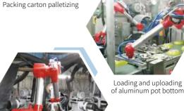
Loading and uploading of aluminum pot bottom
