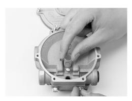
20. Set the secondary spring (9) in its seat on the converter body, then position the secondary lever and fulcrum pin assembly on top of the secondary spring (9). Push down until the fulcrum pin seats and hold in place.
