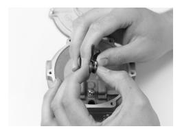
18. Push the nose of the new secondary seat (8) through the hole in the end of the new secondary lever (6).
