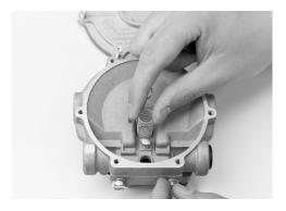
7. Remove the secondary lever (6) and fulcrum pin (7) and retain the fulcrum pin. Remove the secondary spring (9).
