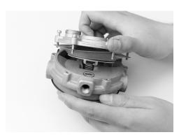
23. Alian the secondary diaphragm (4) to the secondary lever (6) as shown. The end of the lever must protrude through the tab slot on the bottom of the new diaphragm after installation. The screw hole spacing prevents improper positioning secondary diaphragm. 24. Add the secondary cover (3) and install the previously removed screws (2).
