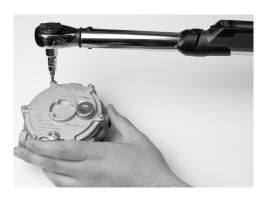
24. Tighten the screws in a crisscross pattern and torque to 22-28 in-lb (2.5-3.2Nm) to complete the installation of the repair kit components.
