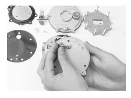
12. Insert the new primary valve pin (13) into the cover plate orifice from the top (converter body side) as shown.
