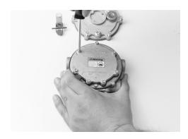
8. Turn the converter over. Remove the seven screws (20) and lift off the primary cover (19).
