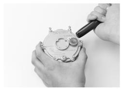
3. Loosen the secondary cover by tapping around the circumference with a plastic screwdriver handle.
