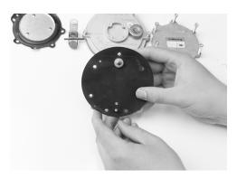
14. Install a new gasket making sure to align the small holes in the gasket to the matching holes in the cover plate.
