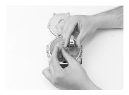
19. Assemble the secondary valve components removed during disassembly. Slide the fulcrum pin (7) through the holes in the secondary lever (6) as shown in the photo.
