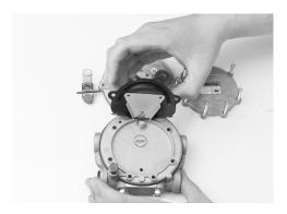
15. Set new primary diaphragm (18) from the kit on the converter body. Screw hole spacing prevents improper orientation of the diaphragm.
