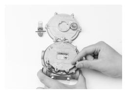
16. Carefully place the primary cover (19) over the diaphragm. Hand-thread the screws (20) through the cover and cover plate into the converter body.
