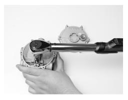
21. Insert screw (5). 22. Tighten screw to 22-28 in-lb. (2.5-3.2 Nm).
