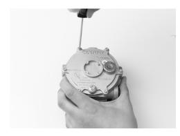
2. Remove the 6 screws (2) from the secondary cover assembly (3).
