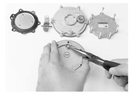
10. Remove the body cover plate (14) and gasket (12) from the body (10). Remove the "E" clip (17) from the primary valve pin (13). Remove the spring (16).
