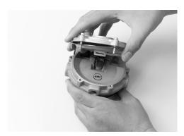
5. This photo shows the secondary cover and diaphragm removed and their orientation to the secondary lever.
