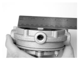
22. Check the secondary lever height. Using a straight edge, the end of the secondary lever should be 1/32" (0.794 mm) below the casting level.
