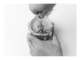
6. Remove the secondary lever fulcrum retaining screw (5).
