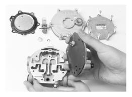
11. Turn the cover plate over and remove the primary valve pin (13). Remove the gasket (12) from the cover plate.
