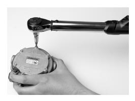
17. Tighten the screws (20) and torque to 22-28 in-lb. (2.5-3.2 Nm) using a crisscross pattern.
