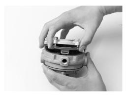
4. Remove the secondary cover (3) and secondary diaphragm (4) as a unit. Note the secondary lever protruding through the metal tab slot of the secondary diaphragm. Slide the cover and diaphragm forward to free the lever from the slotted tab of the diaphragm. Take care not to bend the lever.
