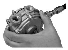
25. Apply 100 psi of air pressure to the inlet side of the regulator and test for leaks. Draw a soap bubble across the regulator outlet to verify that no air is flowing through the outlet. If air escapes, the rebuild has failed and the regulator must be replaced. Actuate the primer button (found on early models) and the soap bubble should burst and air flow should be noted at the converter outlet. Use soap and/or commercial leak detector solution
