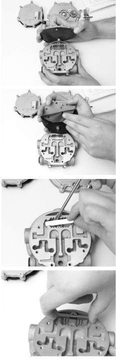
Step 8) Remove cover plate and the gasket.
