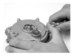
Step 25) Attach a 100 psi air pressure hose to the regulator "INLET" fitting.
