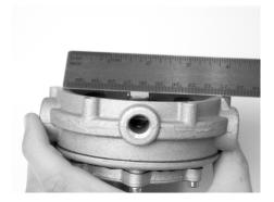
Step 21) The end of the secondary lever should be 1/32" below the level of the body casting. Use a straight edge to measure. Remove and gently bend the lever if necessary to obtain the correct height.
