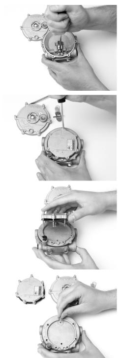
Step 4) Remove the secondary lever fulcrum retaining screw (C-S1-17460-001). Remove the secondary lever and fulcrum pin and set aside for reassembly. Remove the secondary spring.
