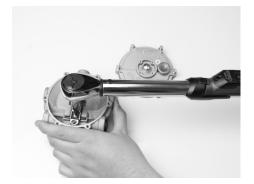
Step 20) Tighten the screw to 32 +/-3 in-lbs. (3.62 +/- 0.34 Nm).
