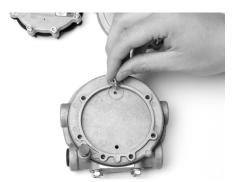
Step 13) Insert the new primary valve pin through the spring and insert into the cover with the larger diameter end of the spring resting against the plate.
