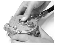
Step 26) For models with a primer button: Depress the primer button several times. Air flow should be detected when the primer is depressed.
