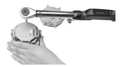
Step 17) Tighten the screws to 22-28 in-lb. (2.5-3.2Nm) in a criss-cross pattern.
