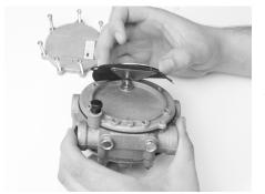
Step 14) Place the cover plate on to the converter body and align the cover screw holes.
