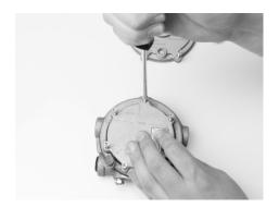
Step 16) Carefully place the primary cover over the diaphragm. Hand-thread the screws through the cover and cover plate into the converter body.
