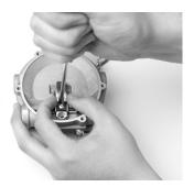
Step 19) Hold the lever assembly with the fulcrum pin in place in its locating groove and fasten in place with the screw (C-S1-17460-001).
