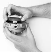
Under normal conditions, installation of a complete Model C-J Repair Kit should be necessary only at the time of a major engine overhaul or when the converter has been out of service for an extended period of time. Each kit includes the necessary gaskets, diaphragms, seals and some replacement screws.
