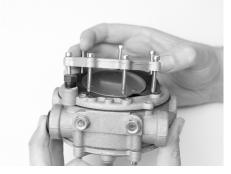
Step 15) Set the primary diaphragm in place on the converter body cover plate. Line up the screw holes to the cover plate.
