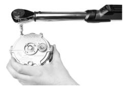
Step 24) Tighten the screws in a crisscross pattern to 22-28 inlb. (2.5-3.2 Nm), to complete the installation of the repair kit components.
