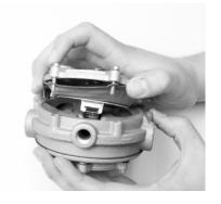
Step 22) Align the secondary diaphragm to the secondary lever as shown. The end of the lever must protrude through the tab slot on the bottom of the new diaphragm after installation. The gap from which the link is punched should be located toward the gas inlet.
