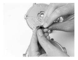
Step 18) Assemble the new secondary seat by inserting the seat retaining tip to the end opening of the lever as shown. Be sure the new seat properly locks into place. Position the secondary spring in place on the body. Place the secondary lever assembly into place over the spring.
