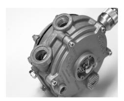
Step 27) Check the primary cover for leaks using liquid leak detector solution. Make sure one of the regulator's secondary outlets is plugged. Draw a bubble of leak solution over the other regulator outlet. The bubble should hold for several seconds when the regulator is pressurized. If any leaks are found, the regulator must be replaced. If no leaks are found, the regulator can be reinstalled and returned to service.
