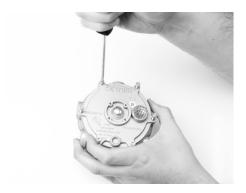
Step 23) Install the secondary cover with the six screws (C-S1-15265-003).
