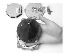
Step 12) Set new primary gasket, (C-G1-85), from the kit on the converter cover plate. The diaphragm will only fit one way (screw hole spacing prevents improper orientation of the diaphragm). The primary pressure hole in the gasket must line up with the hole in the body cover plate.
