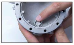
24. Place the seat with the viton (black rubber) side down, in position on jet.
