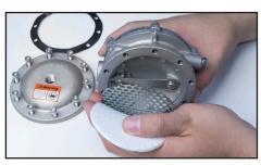
3. Remove C-F1-10 filter and screen C-S7-3.
