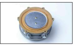
35. Turn diaphragm so the raised lip is downward (see illustration on page 2) place on the Lockoff and rotate to position so the screw hole pattern aligns with the holes in the body (there is only one position in which the holes will line up).
