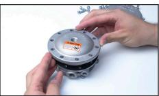
31. Insert screws opposite each other in the "Fuel In" cover and place on gasket. Thread the two screw C-S1-15266-001 through the gasket and into the body.
