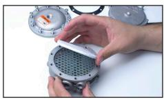
28. Insert C-S7-3 screen and filter C-F1-10 into recess.
