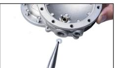
19. Use needle nose pliers to hold C-W1-42 seal retainer washer.
