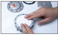
29. Press C-F1-10 filter so that it is properly seated in recess.
