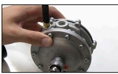
38. Pressurize the "Fuel In" opening with approximately 100 psi of air pressure. Draw a soap bubble across the Lockoff outlet and vacuum port (labeled "VAC") to verify that no air is flowing through either opening. If air escapes, the rebuild has failed and the Lockoff must be replaced. Apply a small amount of vacuum to the port labeled "VAC" to verify the air flows
