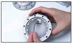
25. C-S2-40 spring ready to be fastened in place. Be sure the arc in the center faces upward (see illustration in step 26 below).
