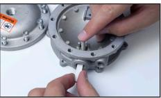
18. Coat the installation pin C-P1-14235 with petroleum jelly and push the seal through the holder and into the seal recess of the C-VFF30 body. Look through the fuel port to ensure the seal is seated in the seal recess and that the groove in the seal is visible.
