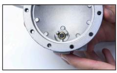
22. Pin C-P1-15 is properly placed in valve jet.
