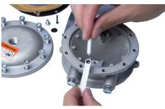
16. Place the C-VFF30 body with the filter side up, as shown in the photo, on a flat surface. Ensure that the groove in the seal is visible from the top of the taper of the seal holder.
