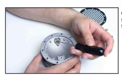
6. Using a small flat head screwdriver, remove C-S4-18 valve seat.
