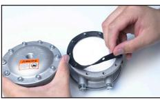
2. Remove cover and C-GI-89 gasket.
