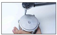
37. Tighten screws alternatively from side to side across cover until all are solidly fastened. Torque to 30 +/-3 in-lbs.
