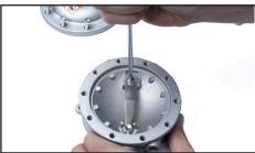
26. Replace spring and fasten in place by C-S1-15265-002 screw (8-32). Align the tip of spring (over valve) and center between the 3 guide fins as shown in illustration. Tighten screw to 30 +/-3 in-lbs.
