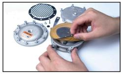
13. Remove cover and diaphragm assy. Clean covers, body and metal parts as necessary with a safety solvent and dry prior to reassembly.
