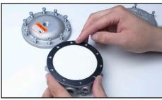
30. Place C-G1-89 gasket in place and align with screw holes.
