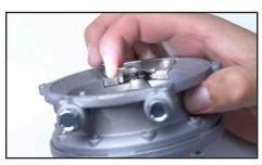
34. Lift lever C-L1-39 to ensure it moves properly and verify that the C-P1-15 lever control pin follows lever travel.
