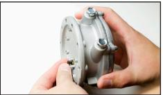
21. Lubricate pin with petroleum jelly and insert through hole in retainer washer and pin lip seal. Again rotate head of pin gently in a circular motion to ease pin into place through washer, lip seal and body housing.
