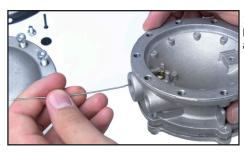
10. Insert paper-clip hook in center hole of C-W1-42 seal retaining washer and remove.
