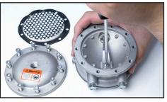
4. Remove C-S1-15265-002 screw retaining valve spring.
