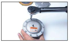
33. Tighten screws, alternating from side to side on opposite sides of the cover until all screws are solidly set. Torque to 65+/-5 in-lbs.
