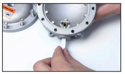
17. Place the holder in the up position and slide the holder into the seal into the body of the C-VFF30. Looking through the fuel port, position the seal above the cavity of the seal recess.
