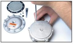
12. Remove 6 screws on diaphragm cover side.
