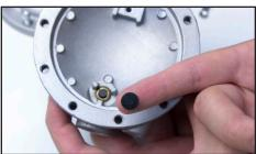
23. Valve seat shown with aluminum side up ready to be placed on jet.
