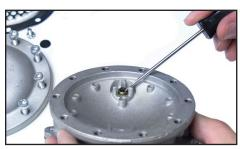
7. Gently lift up and remove the C-P1-15 valve operating pin.
