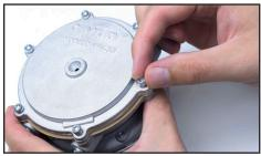
36. Place cover in correct position and insert screws C-S1-15265-001.
