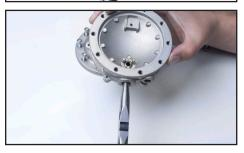
20. Insert seal retainer washer in slot to hold the lip seal in place.
