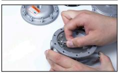
27. When spring is in place, lift slightly to ensure it can move freely.
