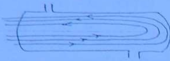
2 Tube Pass & single Shell Pass H.E.
