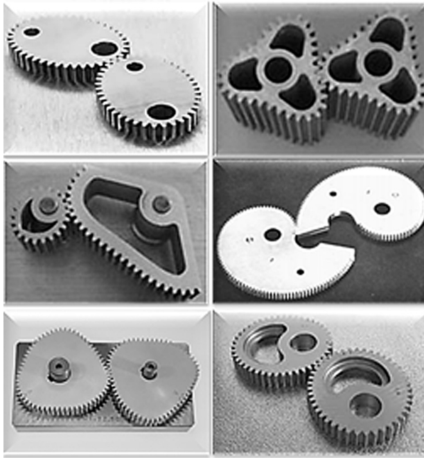
FIGURE 1.13 Various shapes of noncircular gears.
