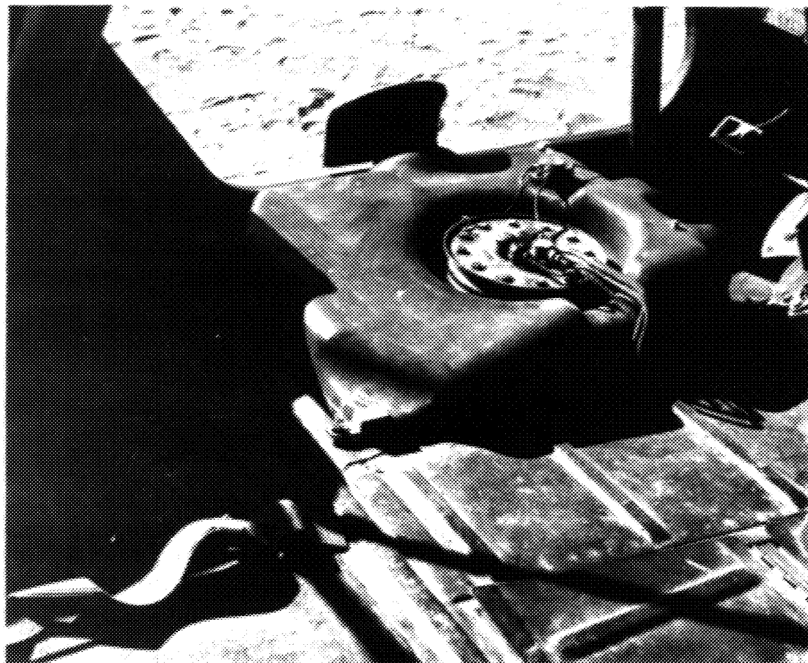
FIGURE 2. Nylon fuel tank as installed in an M151A1 1/4-ton truck (right 3/4 front view)
