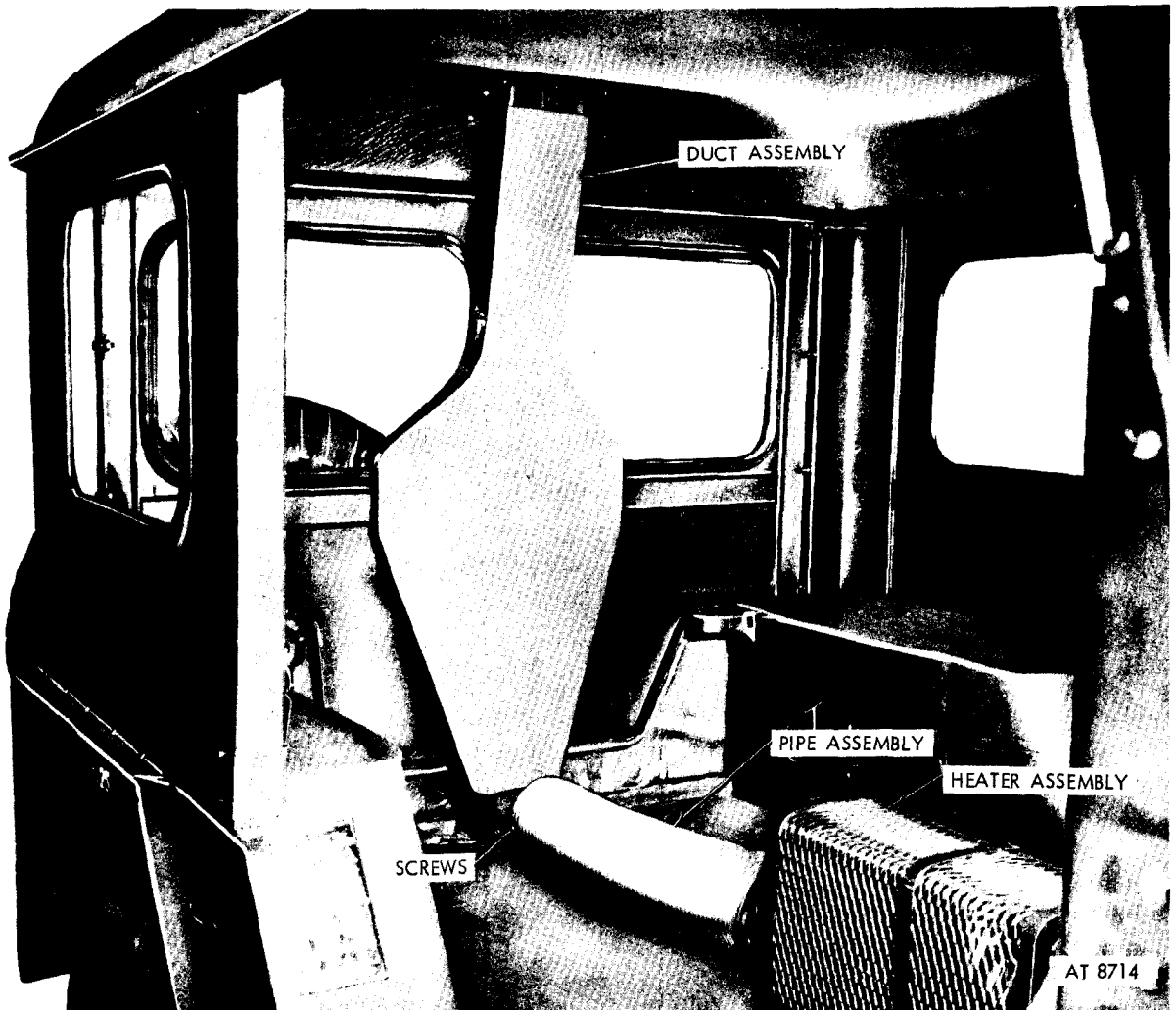
Figure 4-5. Winterization kit (-65° F) duct assembly installed on later model hardtop vehicles.
