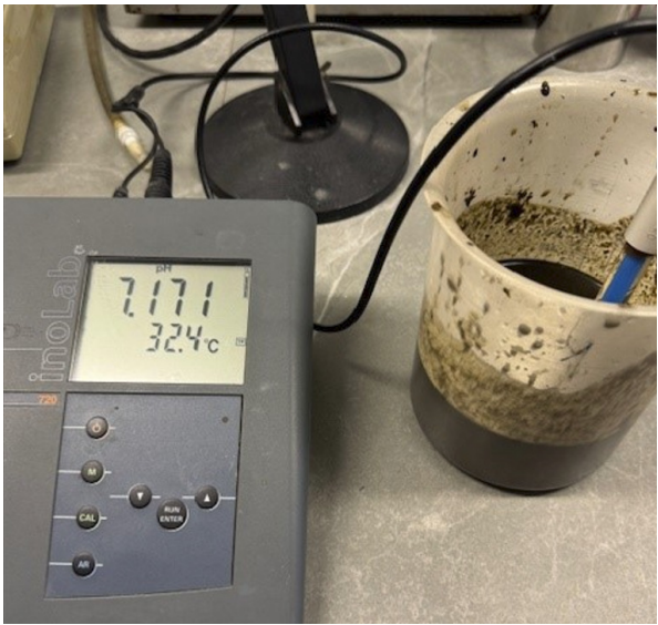
Figure 3.7. Measurement of pH value in the digested substrate from reactor No. 1 (2024-11-10)
