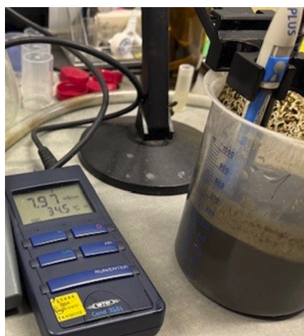
Figure 3.11. Measurement of conductivity value in the digested substrate from reactor No. 1 (2024-11-11)
