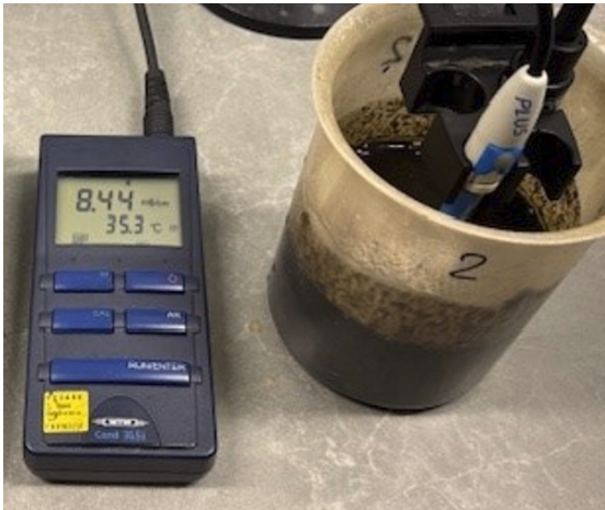
Figure 3.38. Measurement of conductivity value in the digested substrate from reactor No. 2 (2024-12-14)
