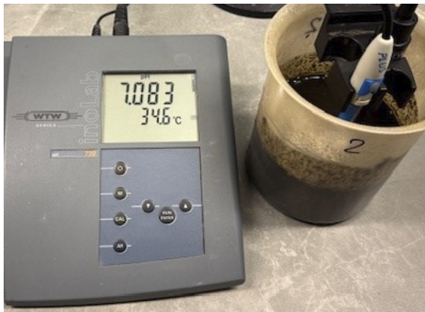
Figure 3.34. Measurement of pH value in the digested substrate from reactor No. 2 (2024-12-14)
