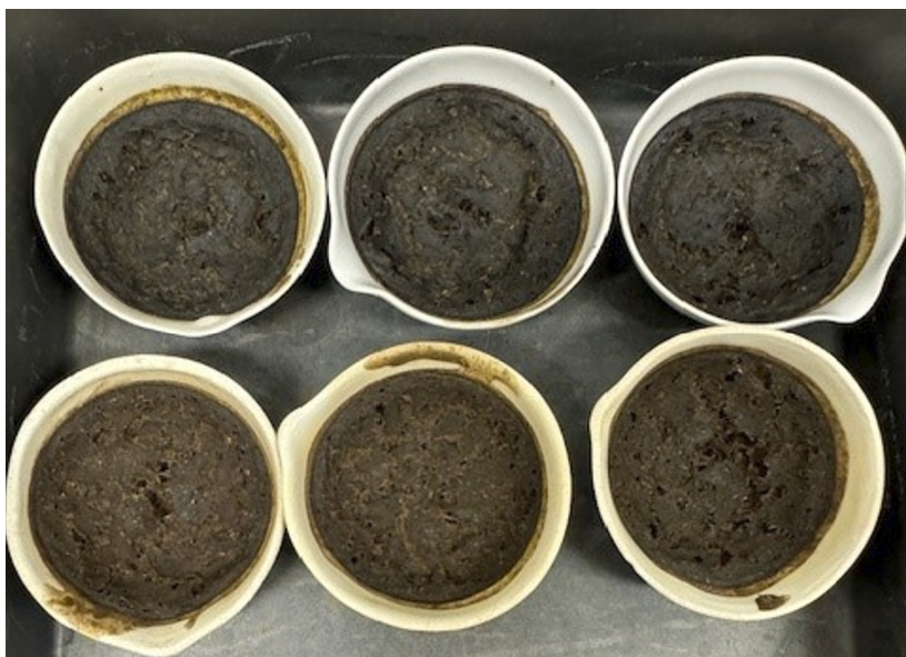
Figure 3.16. Samples of digested substrate from reactor No. 1 (top row) and from reactor No. 2 (bottom row) after drying at 105 °C.
