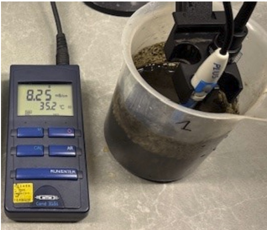
Figure 3.37. Measurement of conductivity value in the digested substrate from reactor No. 1 (2024-12-14)
