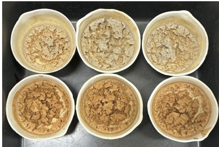
Figure 3.17. Samples of digested substrate from reactor No. 1 (top row) and from reactor No. 2 (bottom row) after heating at 550 °C.
