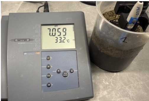
Figure 3.33. Measurement of pH value in the digested substrate from reactor No. 1 (2024-12-14)
