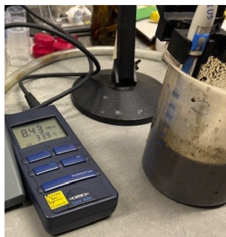
Figure 3.12. Measurement of conductivity value in the digested substrate from reactor No. 2 (2024-11-11)
