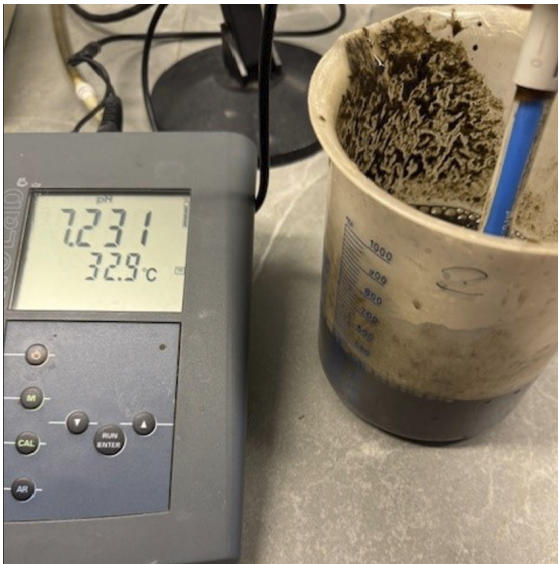
Figure 3.8. Measurement of pH value in the digested substrate from reactor No. 2 (2024-11-10)
