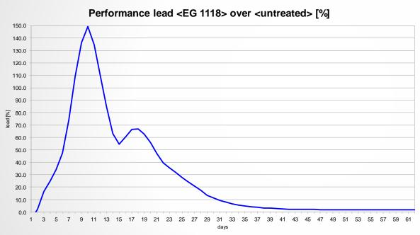
If a short retention time in a reactor is key, the substrate treated with the EG 1118 additive has a significant advantage during the first 30 days. (see above)
