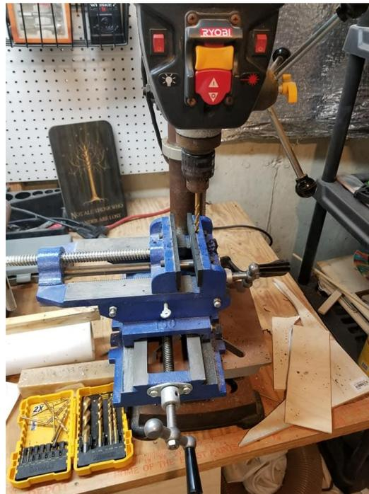
Figure 27 X/Y table mounted to drill press (Brian L. Decker, 2018)
