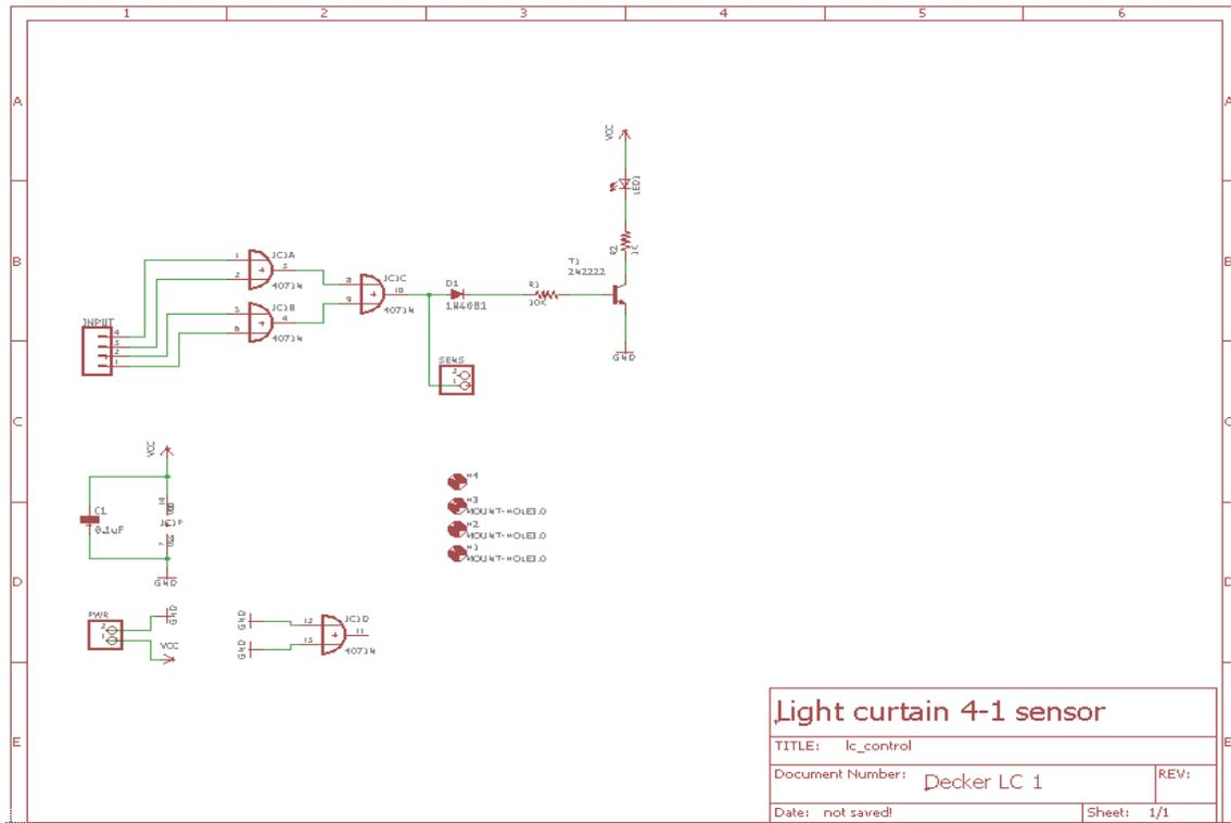
Figure 7 Light Curtain Control schematic (Brian L. Decker, 2018)
