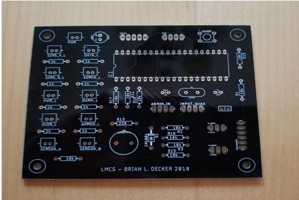
Figure 5 L.M.C.S. PCB initial production sample (Brian L. Decker, 2018)
