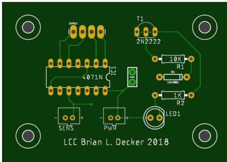
Figure 8 Light Curtain Control PCB – Gerber view (Brian L. Decker, 2018)
