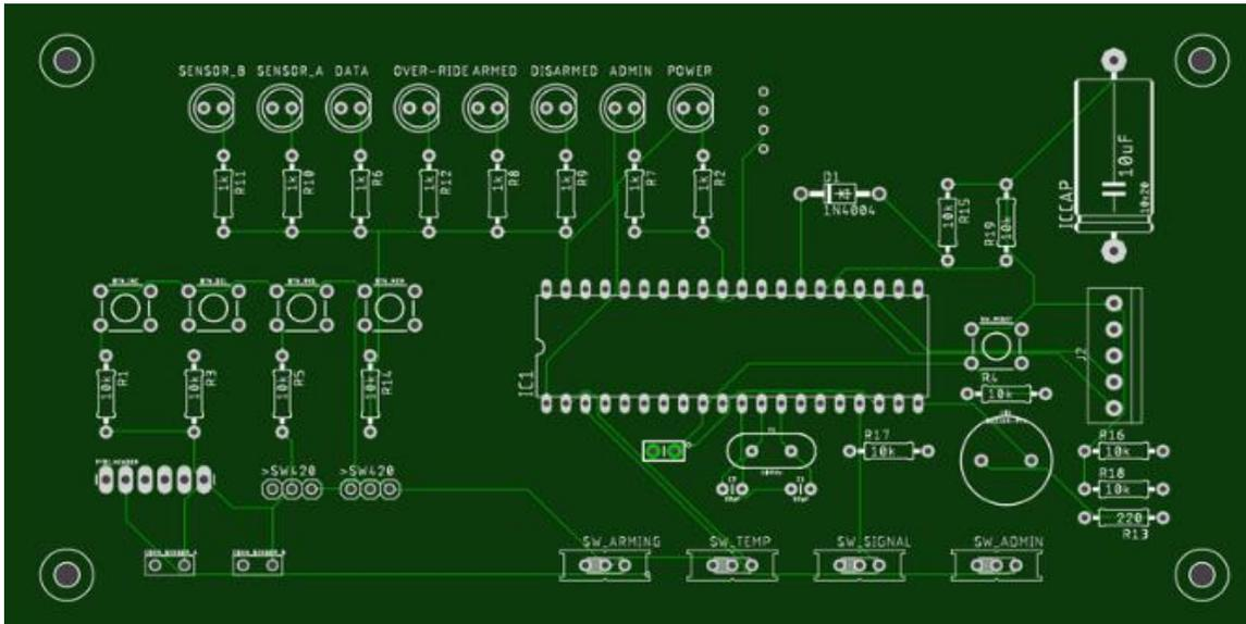
Figure 3 L.M.C.S. initial PCB Layout in SEED Fusion Gerber Viewer (Brian L. Decker, 2018)
