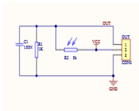
Figure 13 Light Sensor module schematic (OSEPP,2018)
