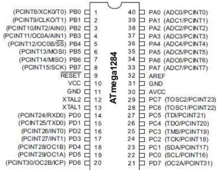
Figure 1 ATmega 1284 Pinout (Atmel Inc., 2018)
