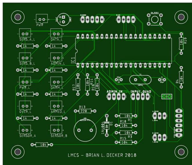
Figure 30 Final L.M.C.S. PCB layout Gerber view (Brian L. Decker, 2018)
