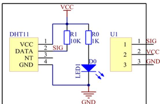
Figure 14 DHT-11 Schematic (OSEPP, 2018)
