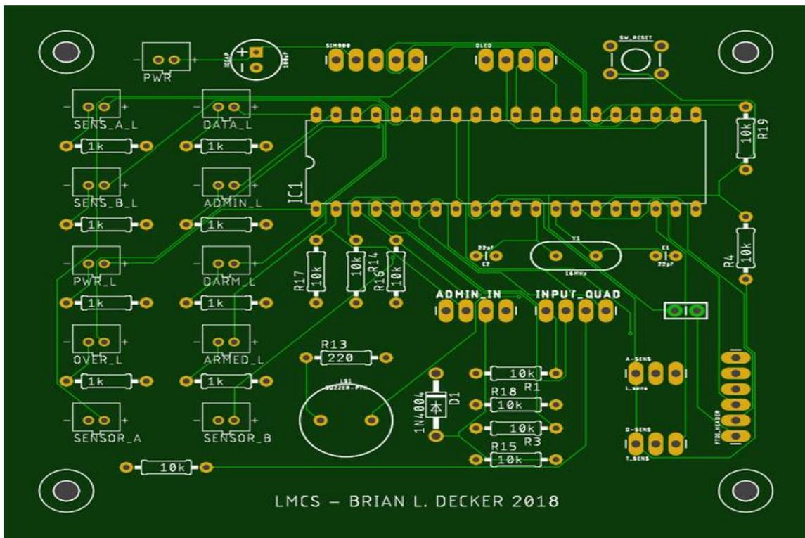
Figure 4 L.M.C.S. PCB Layout 2 in SEED Gerber Viewer (Brian L. Decker, 2018)
