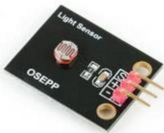
Figure 12 Light Sensor module (OSEPP, 2018)
