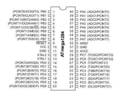
Figure 1 ATmega 1284 Pinout (Atmel Inc., 2018)
