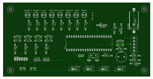
Figure 3 L.M.C.S. initial PCB Layout in SEEED Fusion Gerber Viewer (Brian L. Decker, 2018)
