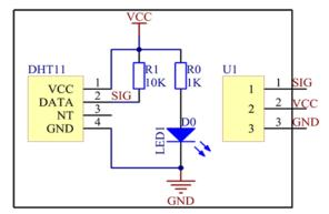
Figure 14 DHT-11 Schematic (OSEPP, 2018)
