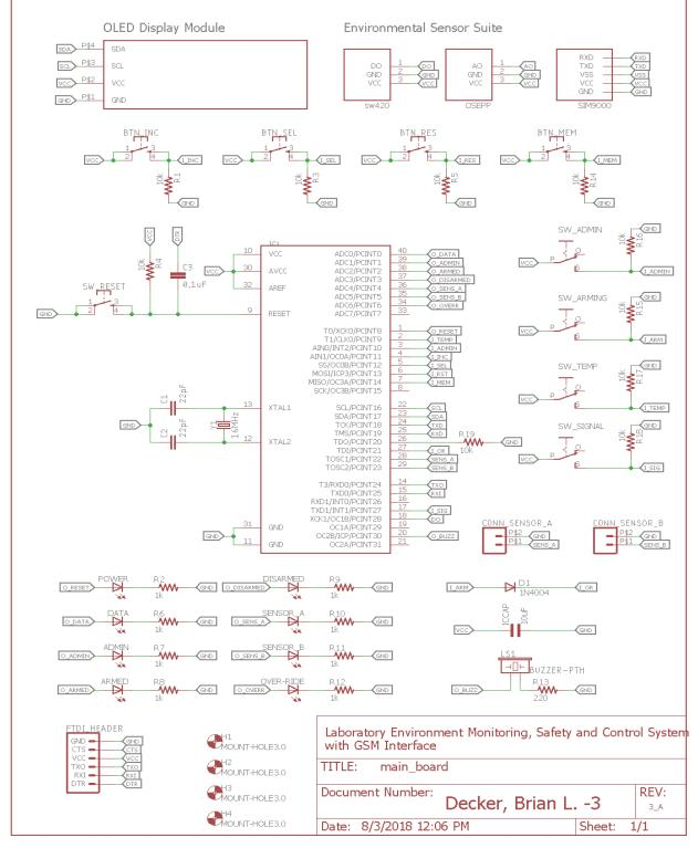
Figure 2 Main Control Schematic (Brian L. Decker, 2018)
