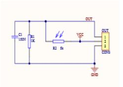
Figure 13 Light Sensor module schematic (OSEPP,2018)
