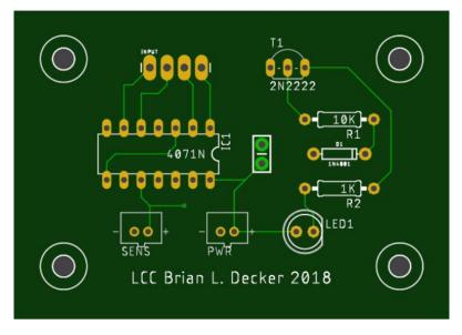
Figure 8 Light Curtain Control PCB – Gerber view (Brian L. Decker, 2018)
