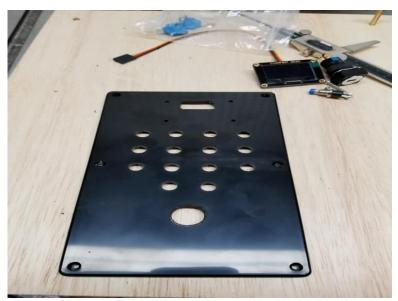
Figure 36 L.M.C.S. faceplate all holes complete and trimmed (Brian L. Decker, 2018)
