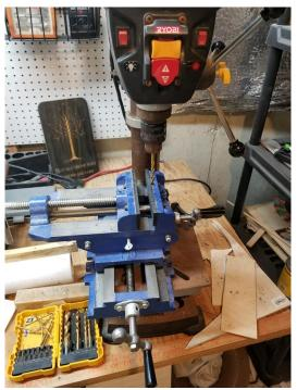
Figure 27 X/Y table mounted to drill press (Brian L. Decker, 2018)
