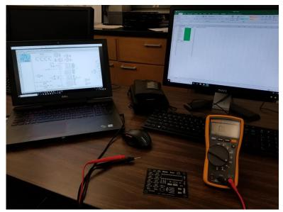
Figure 32 L.M.C.S. testing pad continuity and trace routing (Brian L. Decker, 2018)
