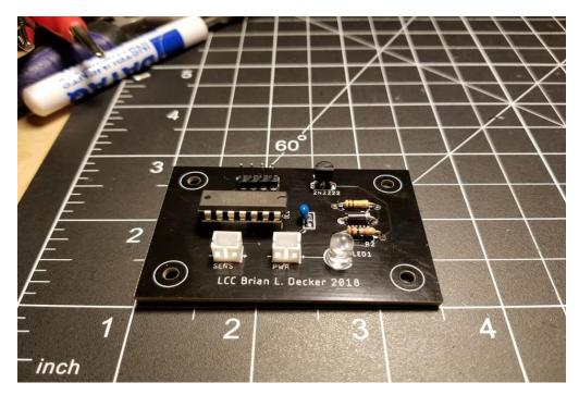
Figure 10 Light Curtain Control PCB – Assembled (Brian L. Decker, 2018)
