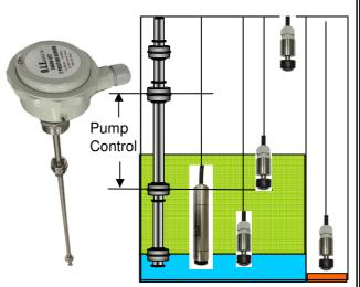
Combined with the T4020 Tank Gauge feeding the inputs of the T4000, the result is a full control system with a single power supply, No floats switches are required in this case, or can be added as fail safe controls.
