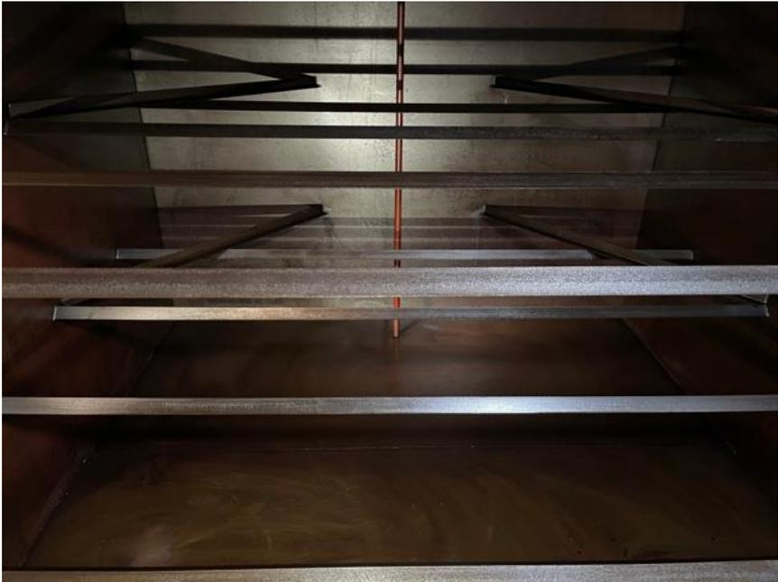
Fig 19. Tank Bracing & Dip Tube
