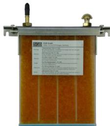
The leak detection unit LDU14 is equipped with a dry filter to avoid condensation and corrosion in the interstitial space. The additional dry filter monitoring FC ensures that the consumption of the dry agent is detected and the spent dry agent is exchanged.
