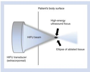
Fig 1 Diagram showing the extracorporeal generation of HIFU and its use to form a thermal lesion within a tissue target.
